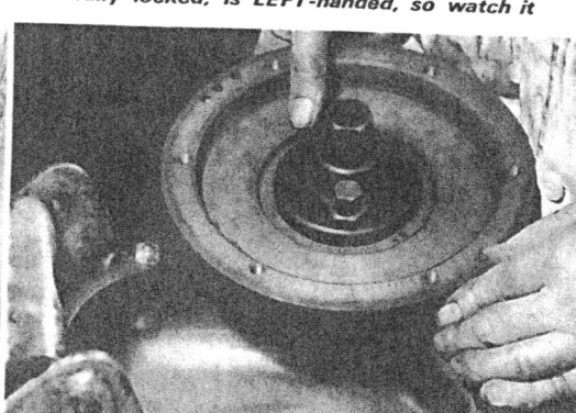
Flywheel is held on a taper, and when it is off, the rear of the engine-case can then be heated to free rear camshaft bearing. If you don't, bearing will stick
